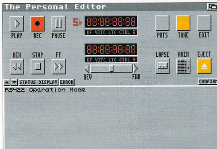
The Nucleus Personal Editor can provide you with precise control over two RS-422 frame-accurate decks with internal time code.
